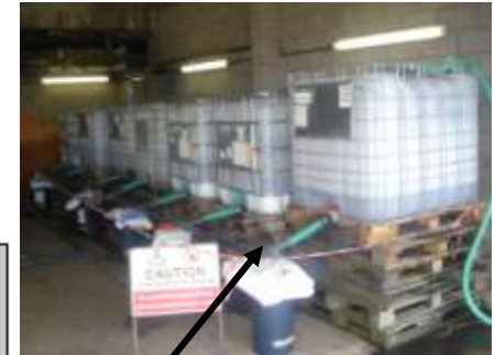
Fig. 1. Pilot-scale struvite crystallizer reactor process design. MAP crystallizer
